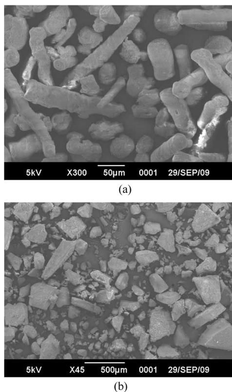
FIGURE 4.—Scanning electron micrographs of (a) HPMC and (b) HPMCA.
