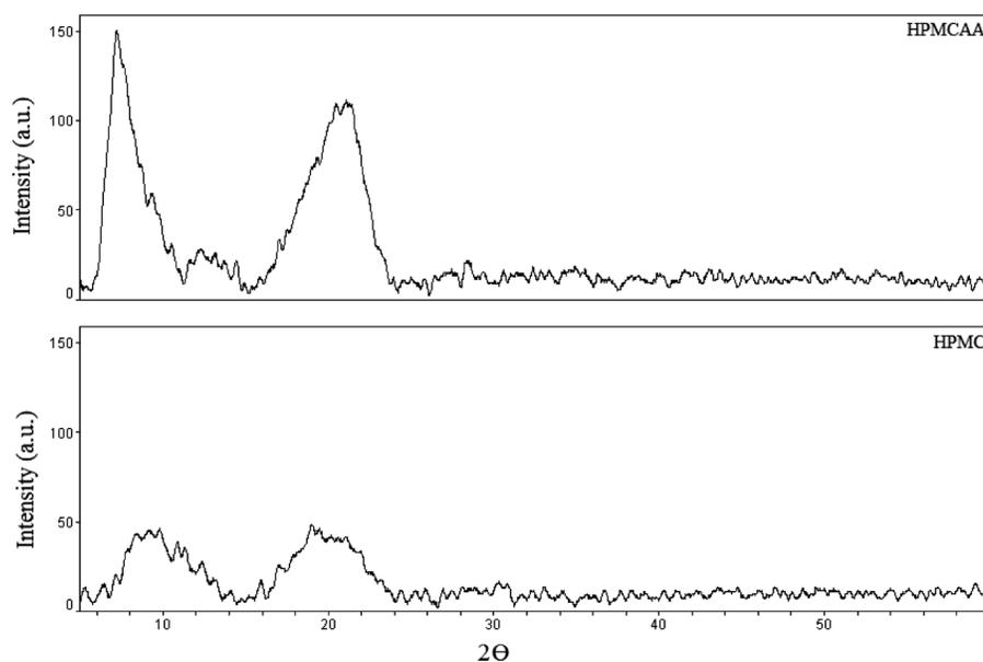
FIGURE 3.—XRD profile of HPMC and HPMCA.
