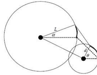
Fig. 3. Relation between motor position and beam angle
