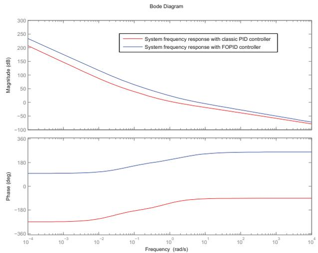
Fig. 9. Comparison of frequency response of ball beam feedback system with integer order PID controller and with fractional order PID controller
