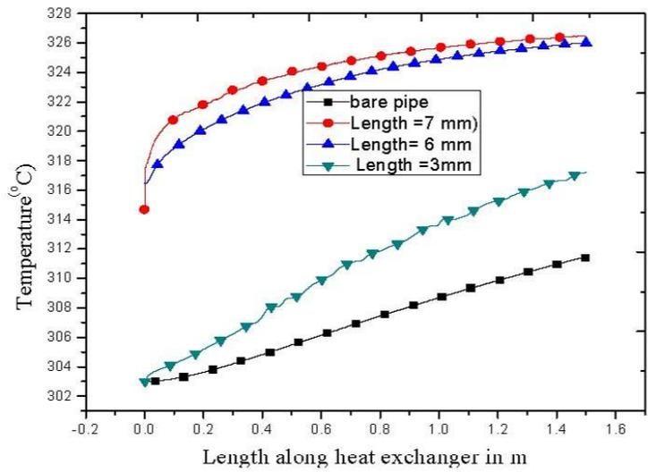
**Fig. 5.** Variation of cold water temperature along the length of exchanger for different heights of rectangular fins for  $mc_h = 0.1$  and  $mc_c = 0.02\text{kg/s}$
