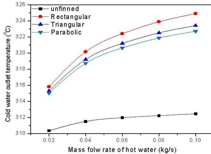
Fig. 9. Variation of cold water outlet temperature with mass flow rates of hot water
