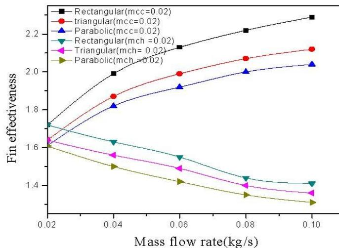
Fig. 13. Variation of fin effectiveness with varying mass flow rates of cold water and hot water
