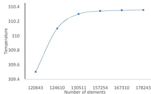
**Fig. 2.** Variation of cold water outlet temperature with number of elements
