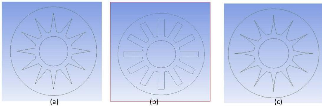
Fig. 7. Different types of finned configurations (a) triangular, (b) rectangular and (c) concave parabolic
