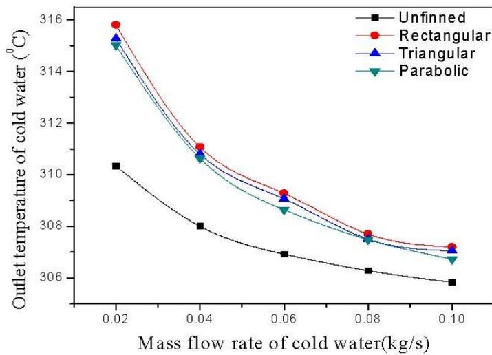
Fig. 11. Variation of cold water outlet temperature with varying mass flow rates of cold water
