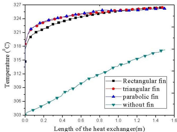
Fig. 8. Variation of temperature along the length of heat exchanger for different fin profiles at  $mc_h = 0.1$  and  $mc_c = 0.02\text{kg/s}$
