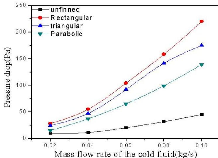
Fig. 14. Variation of pressure drop with varying mass flow rates of cold water
