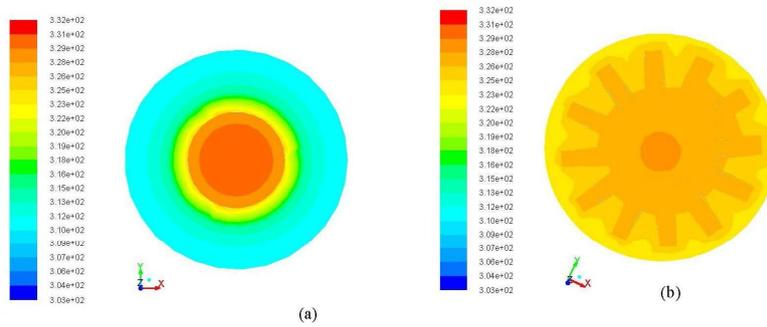
**Fig. 4.** Temperature distribution at the outlet surface for (a) unfinned (b) rectangular finned double pipe heat exchanger (6mm) for  $mc_h = 0.1$  and  $mc_c = 0.02\text{kg/s}$
