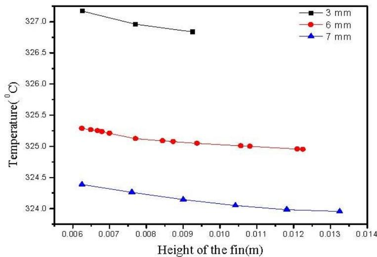
**Fig. 6.** Variation of temperature along the height of fin at the mid-section of the heat exchanger  $mc_h = 0.1$  and  $mc_c = 0.02\text{kg/s}$
