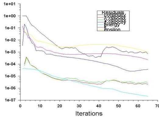
**Fig. 3.** Sample of Residual convergence plot for the double pipe heat exchanger
