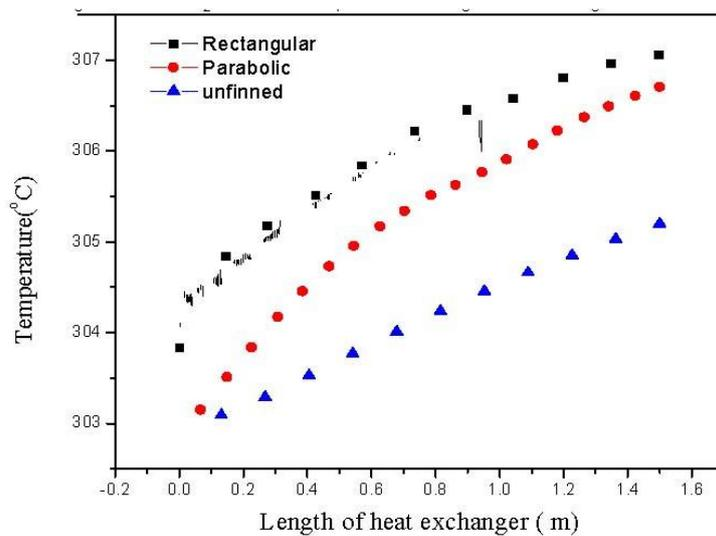
Fig. 10. Variation of temperature along the length of heat exchanger for different fin profiles at  $mc_h = 0.1$  and  $mc_c = 0.02kg/s$
