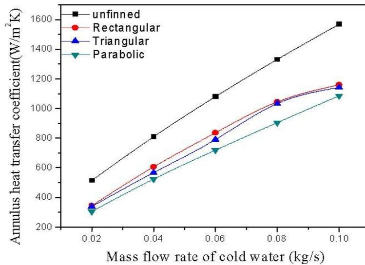
Fig. 12. Variation of annulus heat transfer coefficient with varying mass flow rates of cold water
