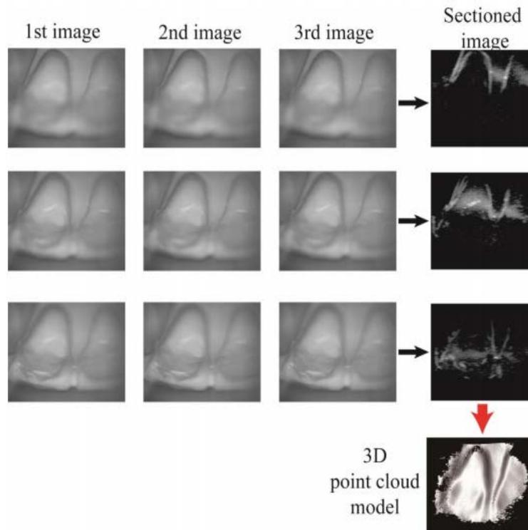
Figure 4d: Optical sectioning from the raw images of the dental cast. The intensity of each pixel of the sectioned image is defined in Equation (1). The sectioned images from different focal planes were stacked to reconstruct a 3D point cloud model of the dental cast
