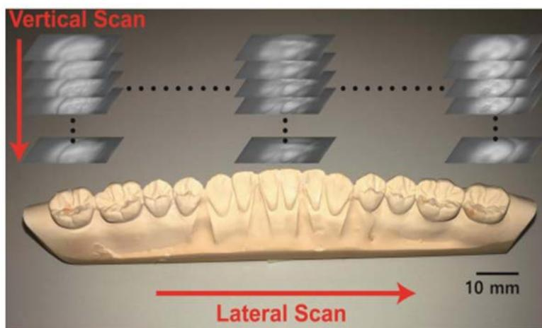
Figure 1: (b) depiction of the dental cast (gypsum model) and the images captured by the scanning apparatus from the top view. Scanning process: Images of the dental cast were listed with different objective lens focal length (vertical scan). The dental cast moved parallelly after each vertical scan was finished (lateral scan). Scale bar: 10 mm.
