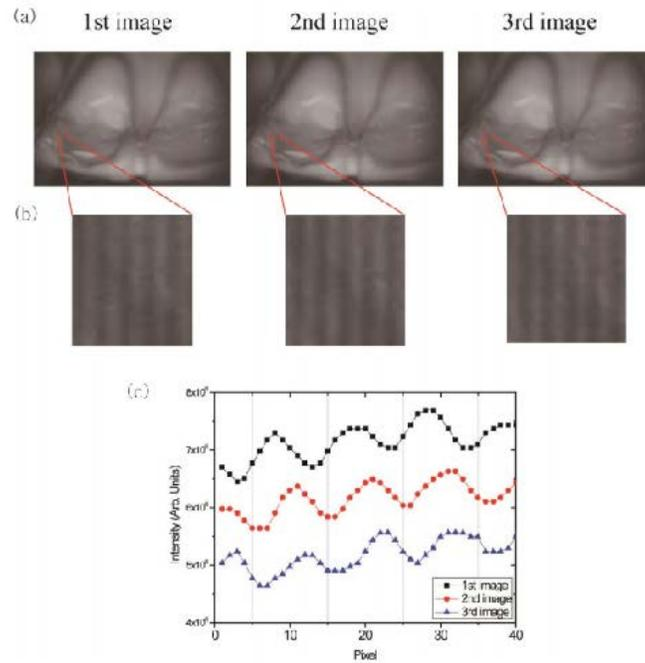
Figure 4: (a) Images (top row) of the dental gypsum cast and (b) magnified images (bottom row) of the in-focus area. Sinusoidal fringe patterns were visualized only within the in-focus areas. (c) The intensity profiles of the magnified images (Figure 4b) along the horizontal axis of the images. The intensity profiles were vertically adapted for better discrimination. The sinusoidal fringe patterns were shifted by  $T/3$  ( $T$ : periodicity of the patterns) between each image.
