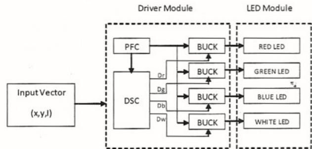
**Figure 2 :** Schematic of RGBW LED source
