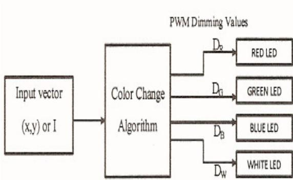
**Figure 1 :** Block diagram of RGBW LED color change algorithm
