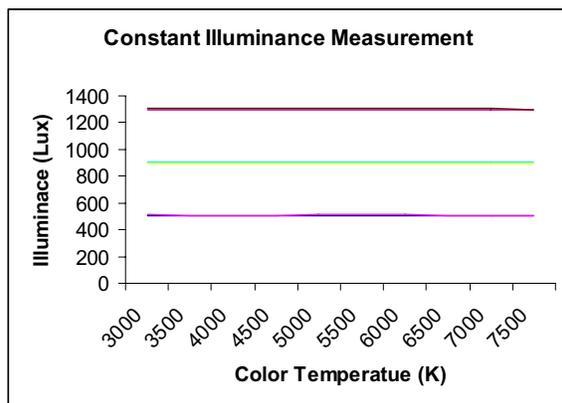
**Figure 3 :** Measuring LED color temperature while maintaing illuminance values constant
