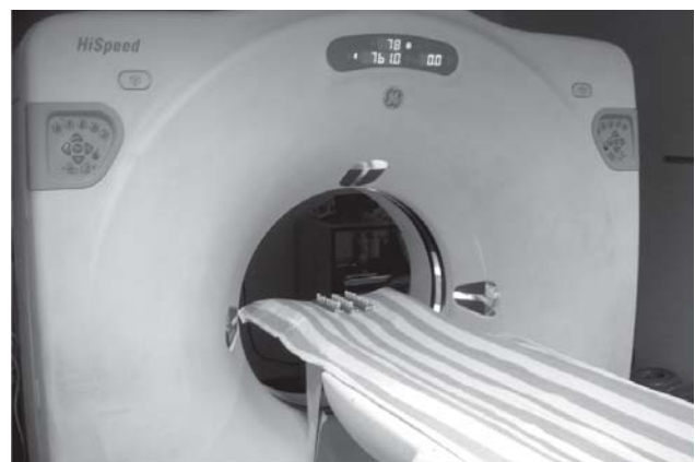
FIGURE 1 - Spiral computed tomography machine used for analysis of the specimens
