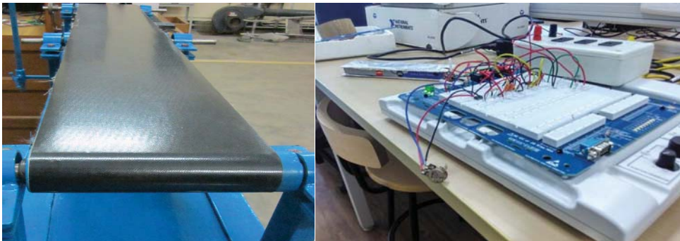
Figure 3. Laboratory setup of a) conveyor and b) sensor and signal conditioning circuit
