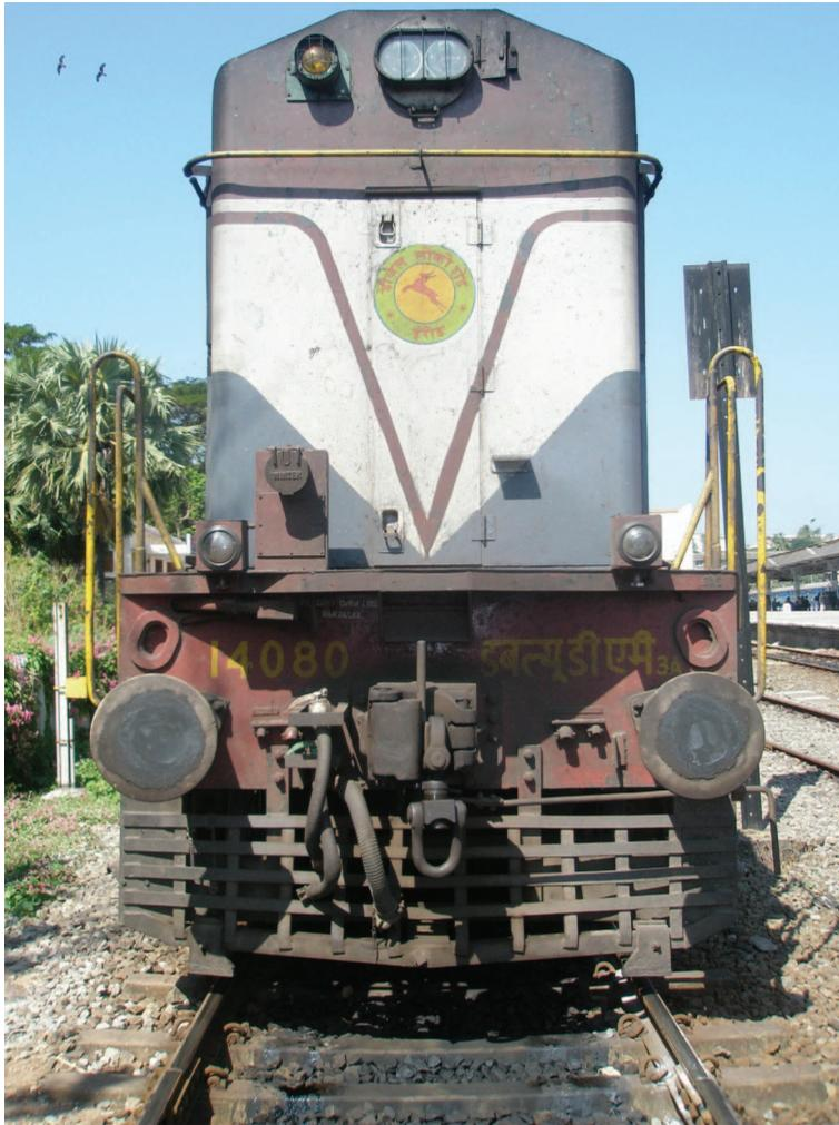
Figure 3. Railway engine showing circular buffers at the corners.
