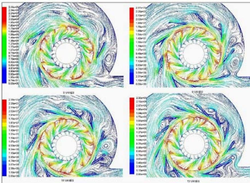
Fig. 6. Instantaneous velocity vector plots for configuration with odd number diffuser vanes.
