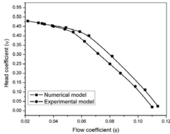
**Fig. 3.** Validation characteristics curve for Head coefficient vs. Flow coefficient
