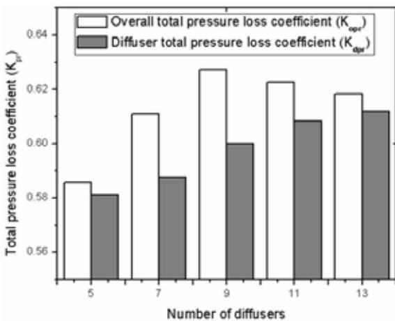
Fig. 10. Total pressure loss coefficient for odd number diffuser vanes.
