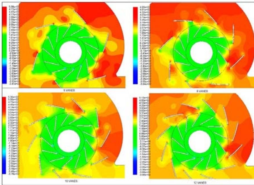
Fig. 5. Static pressure contour plots for configuration with even number of diffuser vanes.
