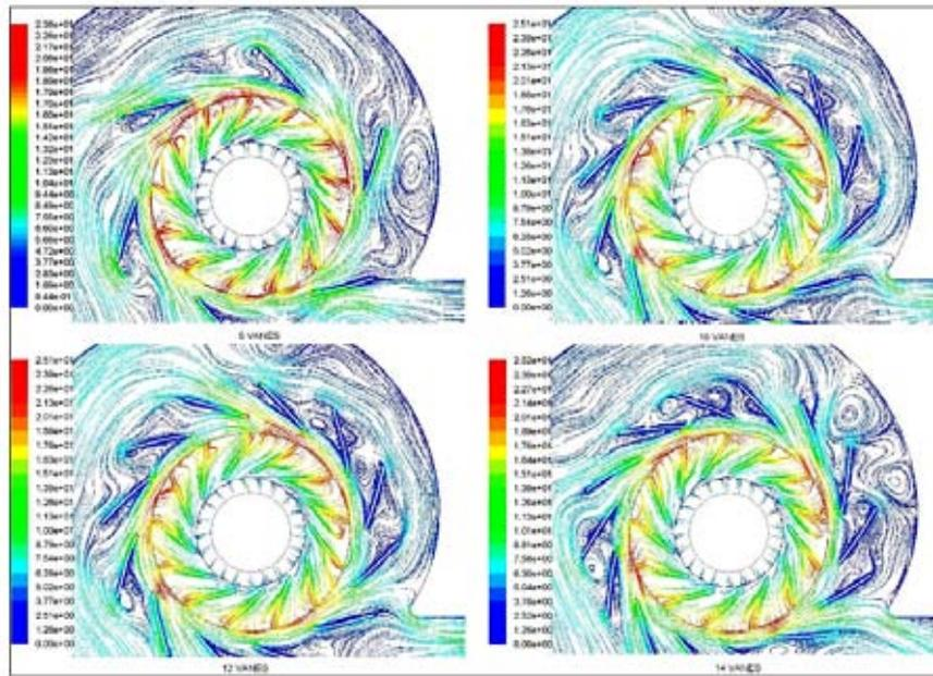
Fig. 7. Instantaneous velocity vector plots for configuration with even number of diffuser vanes.
