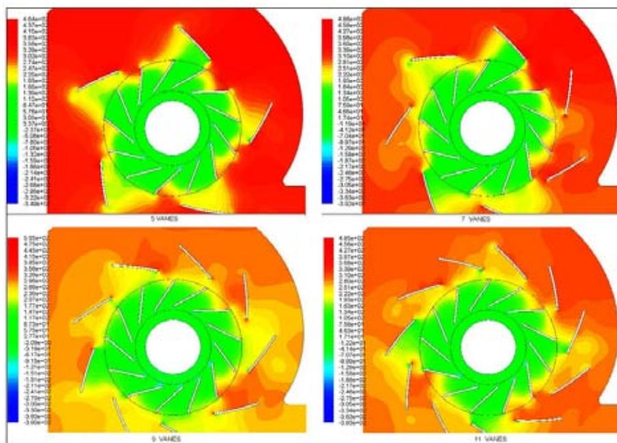
**Fig. 4.** Static pressure contour plots for configuration with odd number of diffuser vanes.
