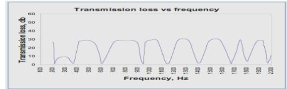
Figure 6b. Plot transmission loss Vs. natural frequency for fixed end condition.
